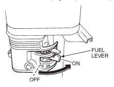
Figure 9. Fuel Valve Lever
